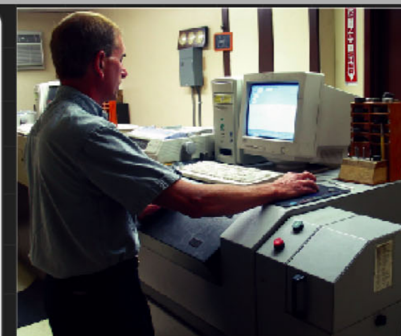
Our direct reading spectrometer give us precise compositional analysis before every pour.
